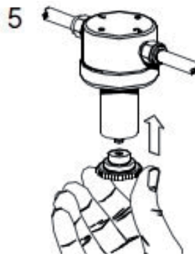
Figure 7 Coalescing Filter Maintenance 3
