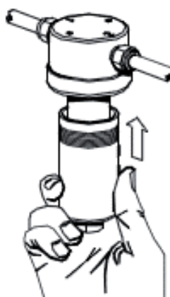
Figure 4 Particulate Filter Maintenance 4
