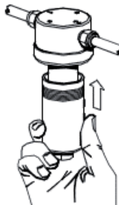
Figure 9 Coalescing Filter Maintenance 5
